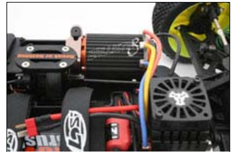
The Ballistic 8 installed in a Losi® 8IGHT-E 2.0 4WD Buggy
